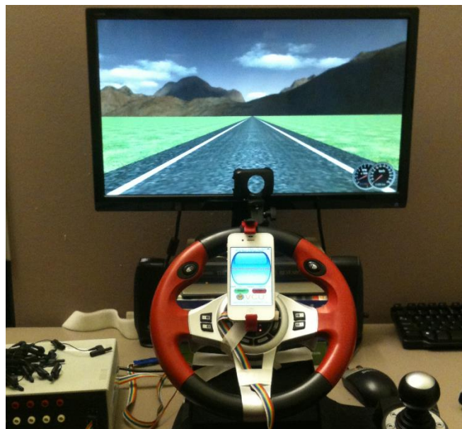
Figure 26. Recording SWM data using an iPhone, an IMU-6050, and a potentiometer.
