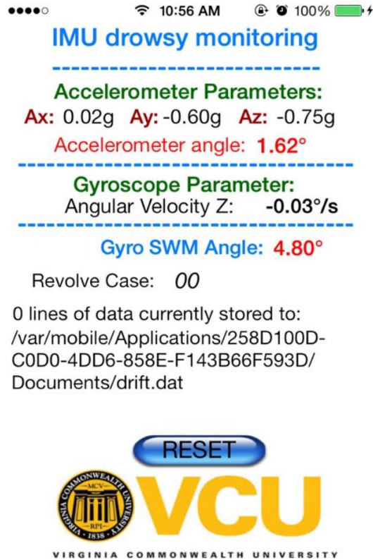
Figure 28. Recording SWM data using an iPhone, an IMU-6050, and a potentiometer. Unfused gyroscope data revealed drift over time
